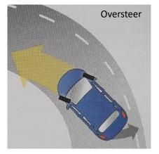
**Note:** Modern vehicles have electronics to minimise the risk of a resulting skid, although Carmakers tend to engineer in Understeer under extreme conditions, it being generally safer to hit an obstacle in front, rather than on the side of the vehicle, as that is where the majority of the impact absorption and safety systems are placed.
