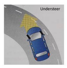
**Understee**r (LEFT) is the tendency of the vehicle to **turn less** in response to a given turn of the steering wheel. Most front-wheel drive vehicles will tend to understeer.
